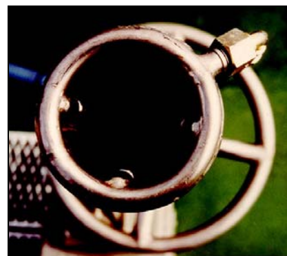
Figure 5 - 39 A close-up view of the PIJESP's suction head showing the nozzles mounted inside the mouth pointing inwards.
