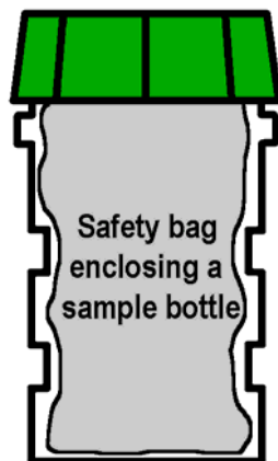
Figure 4 - 16 Plastic jar used as an outer container for the sample bottle which is enclosed in a safety bag.
